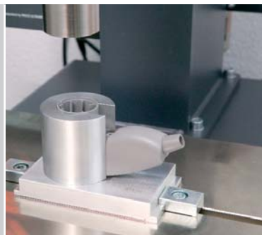
Welding of a thrombectomy system in cleanroom environment
