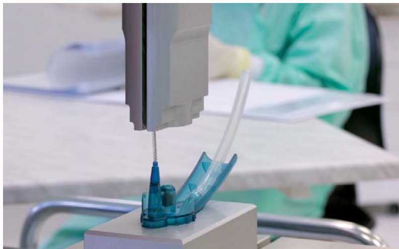
Welding of a thrombectomy system in cleanroom environment
